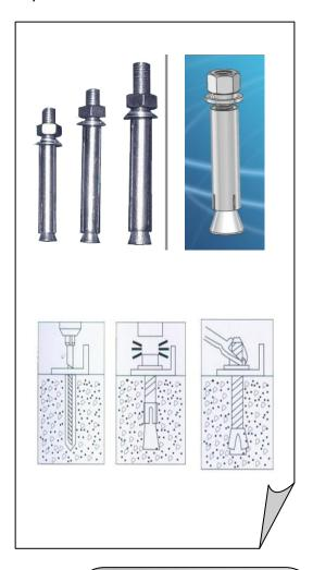
4.2 Concrete ground only need to fix 2\*M12\*100 expand-bolt firstly
