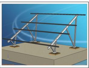
5. Prolong rail or connect rail of two arrays, fix by four M10\*35 bolt
