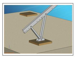
1.2 Fix back feet base to expand-bolt by M12 nuts.
